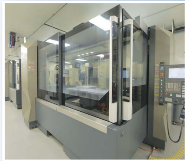
New vertical format mills have been installed as a part of a multi-million dollar re-invention of the Tool Room at Prent's World Headquarters.
